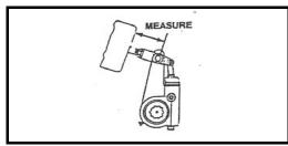
Another person must apply and hold the service brakes with at least 100 p.s.i. in the air tanks.
