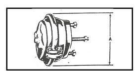
Measure the distance from the bottom of the air chamber to the center of the large clevis pin.
